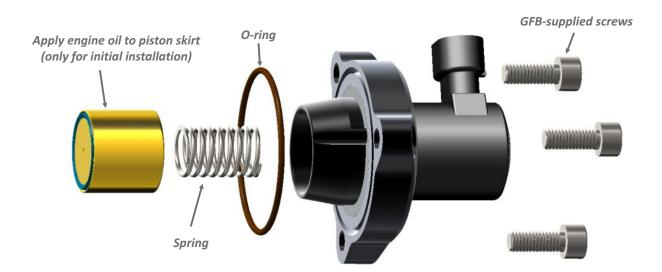
Ensure the DV+ valve body, piston, spring, and o-ring are assembled as shown above, then install the assembly onto the factory mounting location using the supplied screws, making sure to hold the piston during this process to prevent it from falling out.
