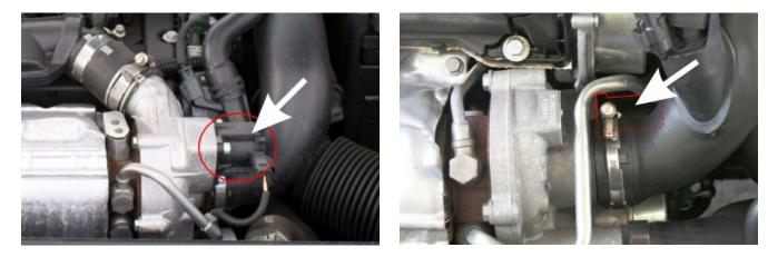
In all cases, begin by removing the intake duct to gain access to the diverter valve and the 3 screws that mount it to the turbo.
