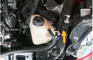
Unclip the electrical connector from the diverter valve ( ), then remove the 3 mounting screws using a 5mm metric hex key. Remove the diverter from the car.
